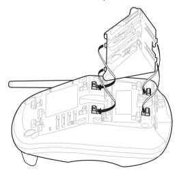
To put the phone on a slant, insert the clips into the middle clip slots. Then, tilt the bracket down so the tabs click into the upper tab slots.
