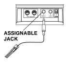
To connect a sustain pedal to your MD-1600, insert the plug on the pedal's cord into **ASSIGNABLE JACK** on the back of the keyboard.
