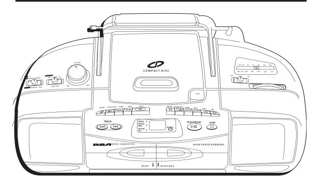
If you know what each button does, it's easy to figure out how to operate the tape decks. PAUSE **II** — Press to interrupt tape play or record mode. Press a second time to resume tape play **STOP/EJECT** ■ — Press to stop current tape activity, or to open the cassette compartment door
