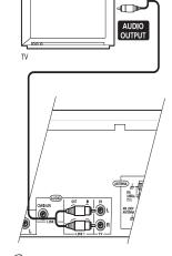
Connect a stereo audio cable (not supplied) from the audio outputs of your TV to the **TV IN** jacks on this system.
