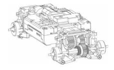
**9** Align the shafts of the rear arms and re-assemble the rear gear case.
