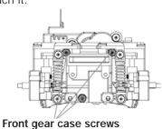
Remove the front center gear and the center shaft and take out the small bearing. Tweezers may be helpful for this step.
