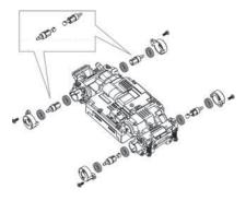
Remove the two screws that hold the rear drive unit and detach it. Remove the upper screw first. Move the rear upper arm and rear attachment holder out of the way, then, remove the lower screw.
