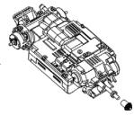
Place the center gear on the center shaft. Lightly press and rotate the center gear so the flat side of the center shaft and the center gear lock together.
