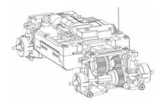
**15** Align the shafts of the rear arms and reassemble the rear gear case.
