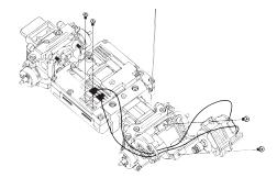
Remove the two screws on the rear drive unit to remove the rear gear case. Then, remove the differential gear and the third gear.
