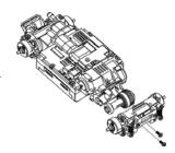
Take out the rear differential gear unit, and replace the bearing on both ends.
