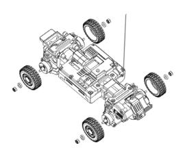
2 Loosen and remove the screw on the knuckle cap (or disk brake if you have changed it). Carefully unlatch the claw on the knuckle cap and pull out the wheel shaft along with the knuckle cap.
