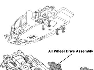
Steps 5 and 6 apply only to cars with an all wheel drive assembly. If you do not have an all wheel drive assembly, proceed to Step 7.
