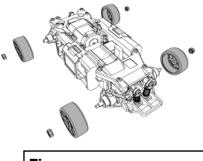
**Tip:** For best performance and fit, before installing bearings, lightly brush each shaft with fine sandpaper to remove burrs and blemishes.
