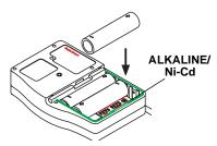
1. Turn the radio off, remove the screw from the belt clip, then slide off the battery compartment cover.
