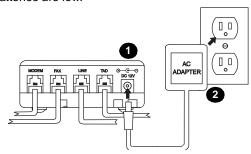
1. Plug the supplied adapter's barrel plug into the AFX-300's **DC 12V** jack.
