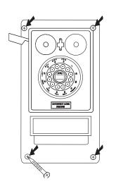
For additional stability, you can also use the supplied rubber spacers in addition to the screws. After you insert the screws through the phone's mounting holes, place a rubber spacer over each screw, so the spacer is between the back of the phone and the wall, then place the phone against the wall
