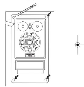
2. Tape the paper "template" on the wall at the desired mounting location.
