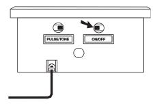
To turn the ringer back on, set (ringer) **ON/OFF** to **ON**.
