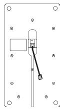
**Note:** If you are not mounting the phone directly over the modular phone jack, press the phone cord into the groove on the back of the phone so the cord is flush with the back.
