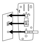
Note: The connector slides up as you slide the phone down so the connection is not broken.
