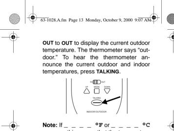
Note: If \_ \_ \_ oF or \_ \_ oC appears, this means that the temperature has exceeded or fallen below the thermometer's measurement range. When the temperature returns to within the measurement range, the display returns to the current temperature display.
