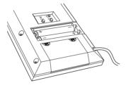
The thermometer beeps and IN, OUT, MAX, MIN, and -188.8° E (test characters) appear, then IN and the indoor temperature appear
