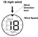
The wind speed and wind direction are updated continuously until the gauge is manually stopped or until it times out (90 seconds). The wind direction icon disappears if no valid direction is received in three seconds.
