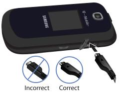
Note: The previous illustration displays the incorrect method for connecting the charger. If attempted, damage to the accessory port will occur therefore voiding the phone's warranty.
