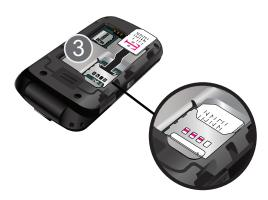
Note: If the card is not inserted correctly, the phone will not detect the SIM card. Remove the battery and re-orient the card back into the slot.
