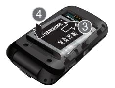
Reinstall the battery cover by sliding it back onto the phone until you hear it securely click. Make sure the battery is properly installed before switching on the phone.
