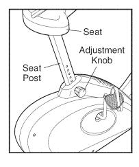
to loosen it (if the knob is not loosened enough, it may scratch the seat post). Next, pull the knob, slide the seat post to the desired height, and then release the knob. Move the seat post upward and downward slightly until the pin on the knob engages one of the holes in the seat post. Then, turn the knob clockwise until it is tight.
