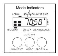
To select the speed, time, distance, fat calories, or calories mode for continuous display, repeatedly press the mode button until the desired mode indicator appears. (Make sure that the scan mode is not selected.)
