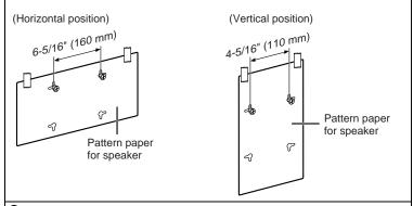
2 Tighten the screws and remove the paper. Hook the speaker on the screw heads and make sure it is secure.
