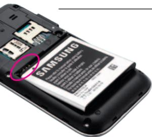
4. Align the gold contacts on the battery with the contacts in the battery compartment. Push the battery into place and replace the battery cover.
