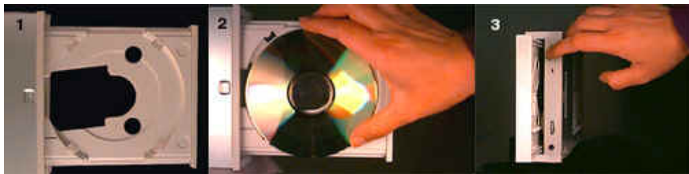
Figure 2. Inserting Disc Vertically
