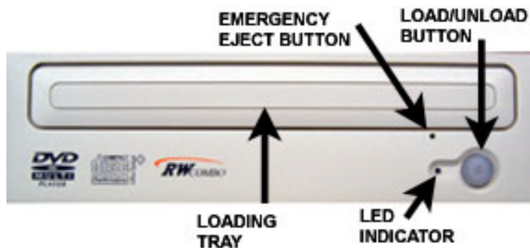
Figure 1.SD-R1612 DVD Writeable Drive Front Panel
