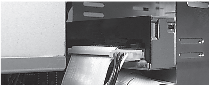
Installing Power Cable
