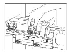
$\mathbf{3}^{\text{ While pushing down on the lever } \textcircled{1}, \text{ pull up the knob}}$
