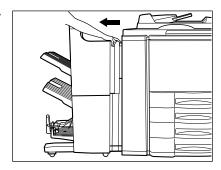
2 Open the cover of the hole punch unit.
