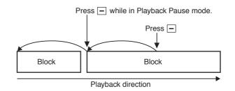
Block shift is also possible during Reverse Playback operation, however playback resumes in the forward direction after the recorded image has been shifted to the head of the desired block.
