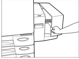
Open the feed-side cover of the automatic document feeder and remove any misfed original.
