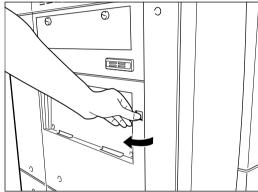
Lower the lower guide of exit side and remove any misfed paper.
