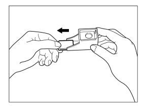
Slide the new staple cartridge fully into the stapler.
