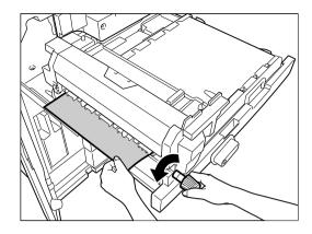
Open the fuser cover and remove any misfed paper.
