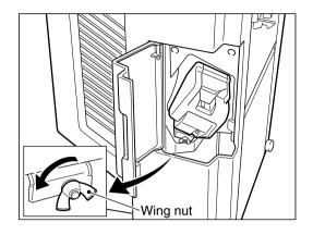
Holding the stapler unit as shown, lift its outer side slightly (arrow ①) and take it out slowly toward you (arrow ②).
