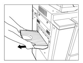
• If a staple sorter is attached, first pull it away from the copier by lifting the release lever.
