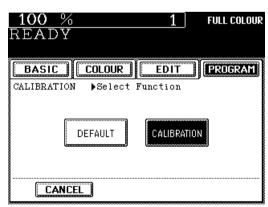
Press the TEST PRINT key to print out the chart for calibration.
