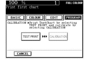
When the display on the right appears, set the chart face down on the glass and with its bottom toward you and its top left aligned against the original scale on the left side, in order that the black line comes to the left side.
