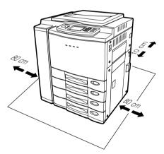
The copier should be located near a wall outlet which should be easily accessible.
