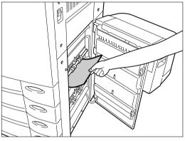
Open the large-capacity feeder cover slowly and remove any misfed paper from inside.
