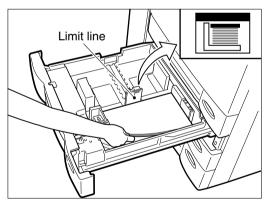
**Note:** Check that there is a slight gap (about 0.5 mm) left between the paper and each of the side guides as shown; the total gap should not exceed 1 mm. If the gap is not suitable, paper misfeeding may possibly occur.
