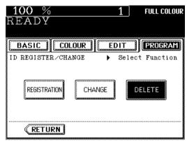
Using the digital keys, enter the access code (4 digits) you want to delete, then press the SET key.
