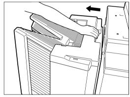
Pull open the paper transport guide of the staple sorter and remove the misfed paper.
