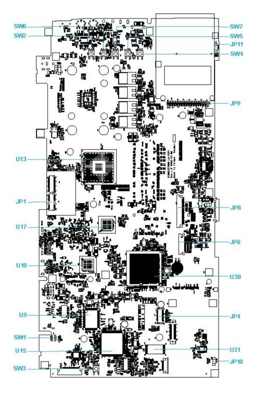
Figure B-2 System board (FRDSY\*) layout (Top)
