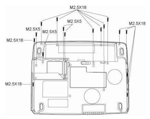
*Figure 4-23 Removing the top cover-2*
