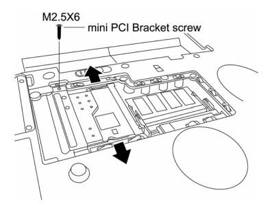
Figure 4-10 Removing the wireless LAN unit
