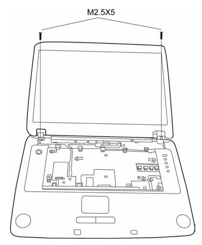
Figure 4-19 Removing the display assembly screws
