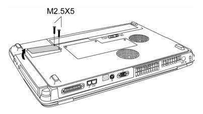
*Figure 4-5 Removing the HDD door*
