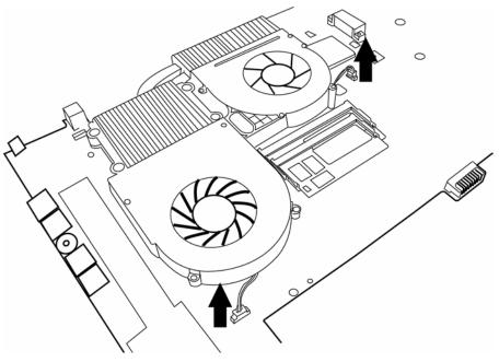
*Figure 4-30 Removing the fan module*
