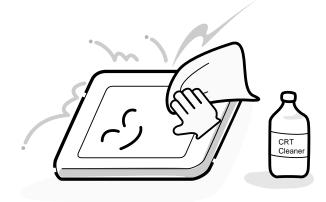
4. If water or other liquid is left on the panel's surface for a long period, it can change the screen's tint or stain it. Be sure to quickly wipe off any liquid.
