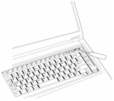
Figure 4-14 Removing the strip cover
