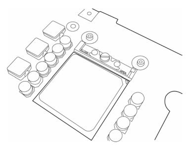
Figure 4-32 Removing the CPU
