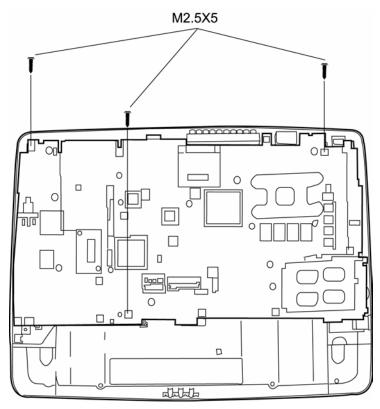
Figure 4-27 Removing the system board
