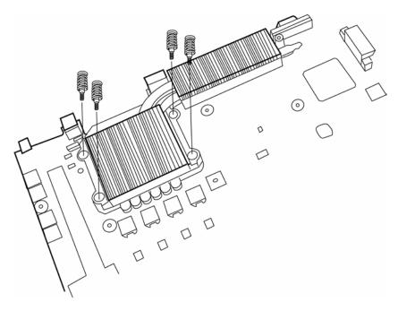
Figure 4-31 Removing the heat sink
