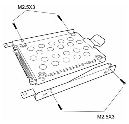
*Figure 4-6 Removing the HDD bracket*
