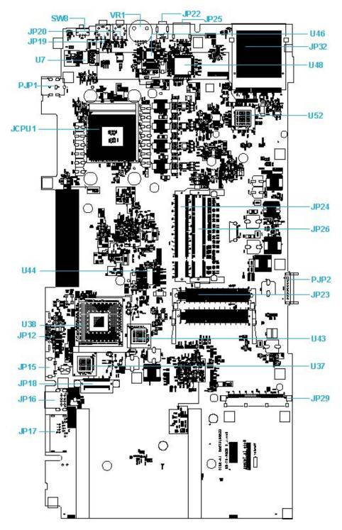
Figure B-1 System board (FRDSY\*) layout (Bottom)
