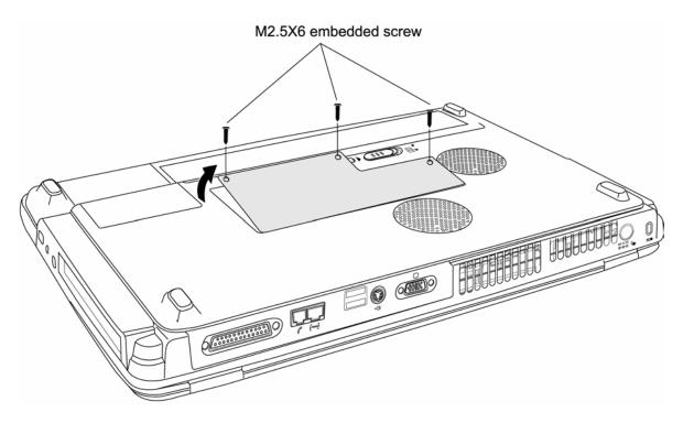
*Figure 4-12 Removing the expansion memory cover*
