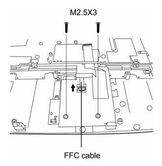
Figure 4-24 Removing the Touch Pad LED board
