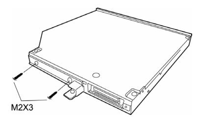
*Figure 4-8 Removing the optical drive bracket*
