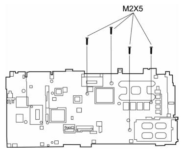
Figure 4-29 Removing the fan module screws
