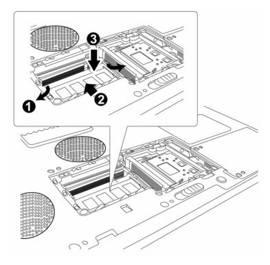
Figure 4-13 Installing the expansion memory
