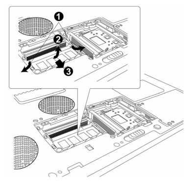
*Figure 4-11 Removing the expansion memory*
