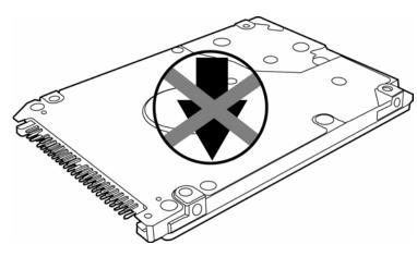
**NOTE:** When handling the HDD, do not press the top surface as shown by the arrow. Hold it by the sides.
