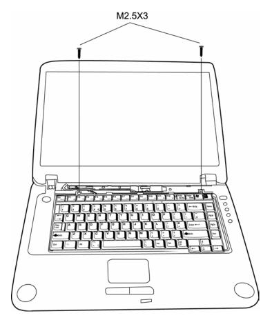
*Figure 4-15 Removing the keyboard*
