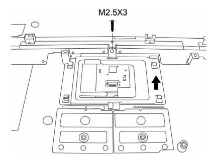
Figure 4-25 Removing the touch pad
