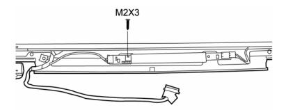
Figure 4-36 Removing the FL inverter board
