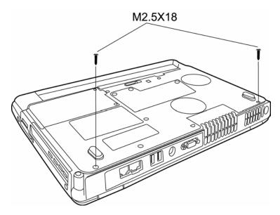
Figure 4-18 Removing the display assembly screws
