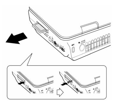
*Figure 4-2 Pressing the eject button*
