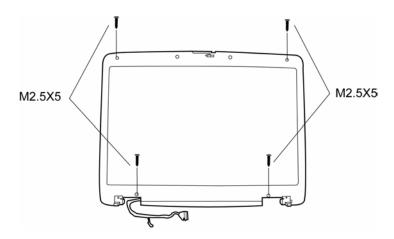
Figure 4-33 Removing the display mask
