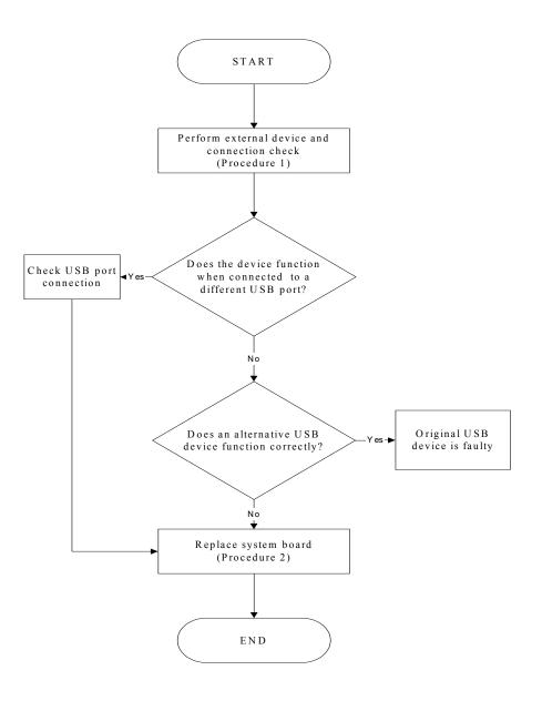
Figure 2-6 External USB device troubleshooting process
