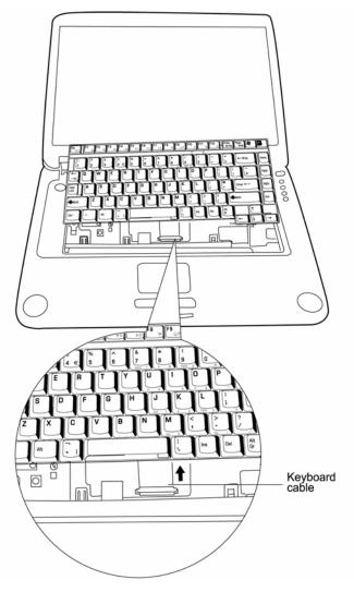
Figure 4-16 Disconnecting the keyboard cable
