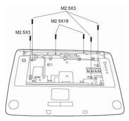
Figure 4-22 Removing the top cover-1
