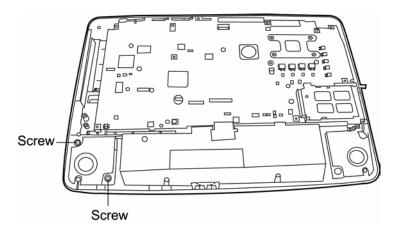
Figure 4-26 Removing the speakers
