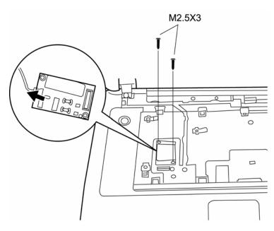
*Figure 4-17 Removing the modem module*
