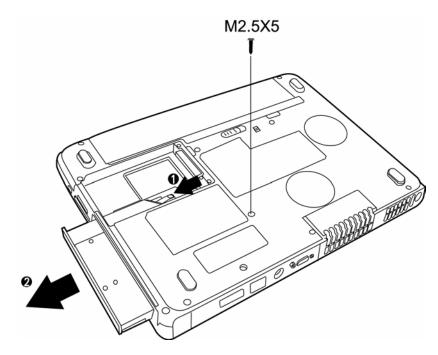
*Figure 4-7 Removing the optical drive module*
