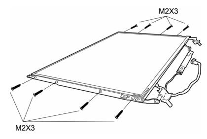
Figure 4-35 Removing the LCD module-2
