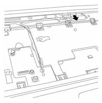
Figure 4-20 Removing the LCD display cable
