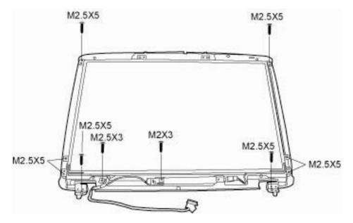
Figure 4-34 Removing the LCD module-1
