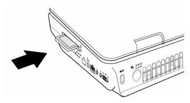
Figure 4-3 Installing the PC card
