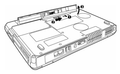
*Figure 4-1 Removing the battery pack*
