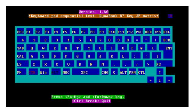
Pressing a key also reveals that key's **scan codes** in the upper right hand corner of the screen. When the key is depressed, its **make code** is displayed. When the key is released, the **break code** is shown.
