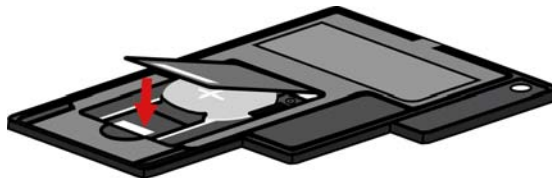
Figure 2-18 Closing the battery cover
