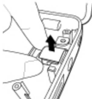
Figure 4-33 Removing DC in cable
