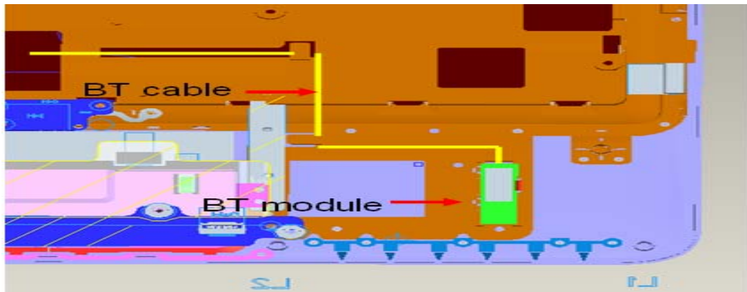
Figure 4-19-1 Remove the Bluetooth cable
