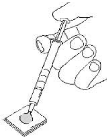
Figure 4-28 Applying silicon grease
