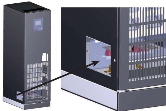
Figure 11-4 - 431B Cable Access Plate
