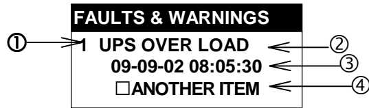
Figure 18 - Warning Screen Example.
