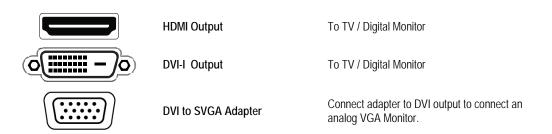
Attach the monitor or monitors to the rear of the recorder using the cable supplied by the monitor manufacturer. Refer to the monitor manual for detailed information on how to setup and use it.
