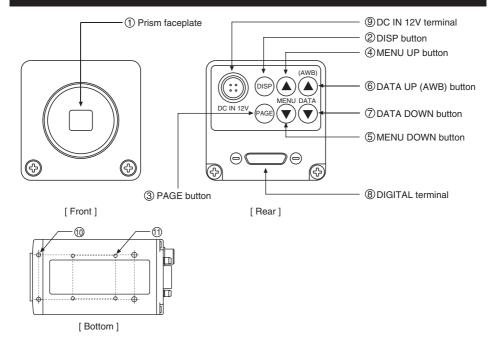
① Prism faceplate The protection cap is attached on the lens mount portion. After removing the cap,
