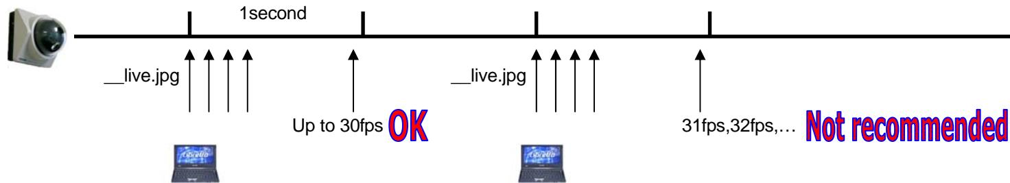
Up to 30fps at 640x480(VGA)/320x240(QVGA)/160x120(QQVGA) resolution
