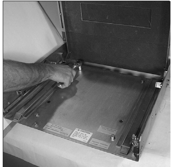
Fig. 11 Fastening Cell to Compartment Floor or Shelf
