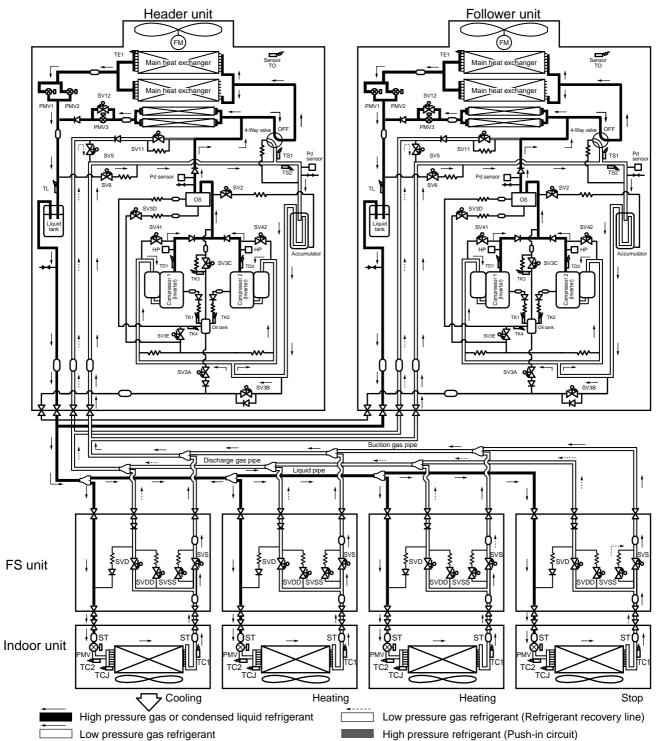
Defrost operation is carried out during all heating operation or Mainly heating, part cooling operation.
