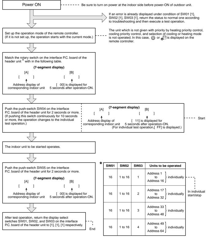
**NOTE)** The individual test operation returns to the normal operation after 60 minutes.
