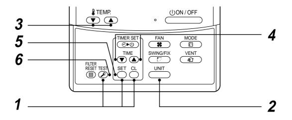
Push SET, CL, and EST buttons simultaneously for 4 seconds or more. The firstly displayed unit No. indicates the master indoor unit address in the group control. In this time, the fan of the selected indoor unit is turned on.
