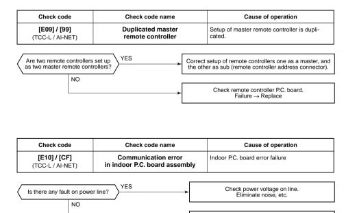
Check indoor control P.C. board. Failure  $\rightarrow$  Replace
