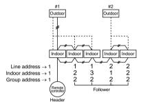
In the above example, under condition of no inter-unit wire of the remote controller, set the address after individual connecting of the wired remote controller.
