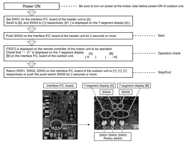
NOTE) The test operation returns to normal operation after 60 minutes.
