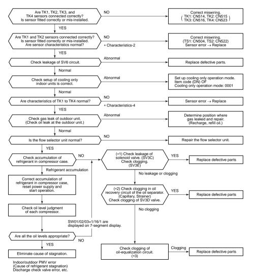
In some cases, it may be difficult to check for leakage or clogging of refrigerant in low ambient temperature condition. In this case, it may take longer for the system to warm up before commencing checks. (Criteria: Discharge temperature of TD1 and TD2 are 60°C or higher)
