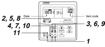
**1** Push simultaneously  $\stackrel{\text{set}}{\bigcirc}$  +  $\stackrel{\alpha}{\bigcirc}$  +  $\stackrel{\text{rest}}{\nearrow}$  buttons for 4 seconds or more.
