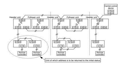
Turn on the indoor/outdoor power of which address is to be cleared. After approx. 1 minute, check that "U.1.- --" is displayed, and then execute the following operation on the interface P.C. board of the header unit of which address is to be cleared in the refrigerant line.
