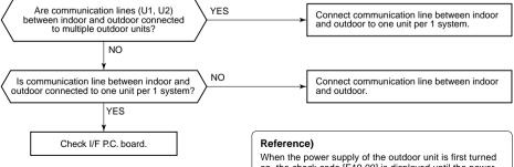
When the power supply of the outdoor unit is first turned on, the check code [E19 00] is displayed until the power supply of the indoor units are turned on. However is not an error. When the power supply of the indoor units are this turned on, the check code is automatically reset.
