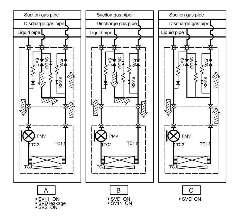
Reference Refrigerant circulating example of flow selector unit when a trouble occurred
