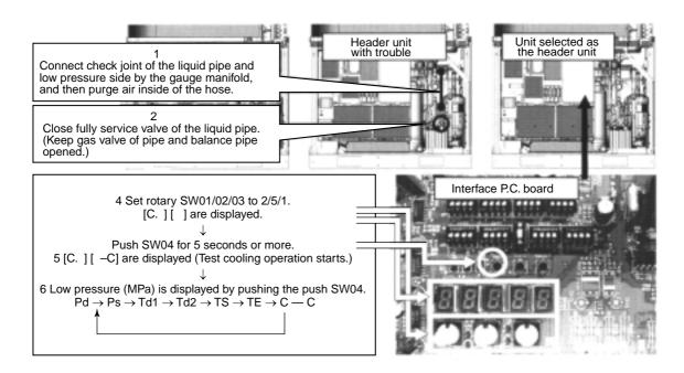
6. Fully close the service valve of the gas pipe on the malfunctioning outdoor unit approximately 10 minutes after the system has started.
