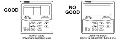
If a frame is not displayed as shown in the above right figure, the power of the remote controller is not normally turned on. Therefore check the following items.
