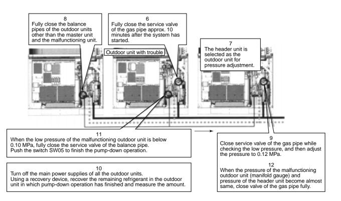
Return all SW01/02/03 of the header unit to (1/1/1) to complete the work.
