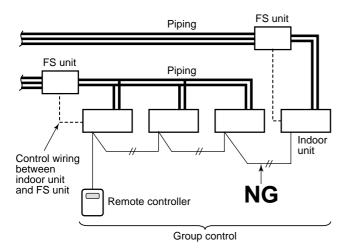
Indoor units off of a single FS unit cannot be individually controlled.
