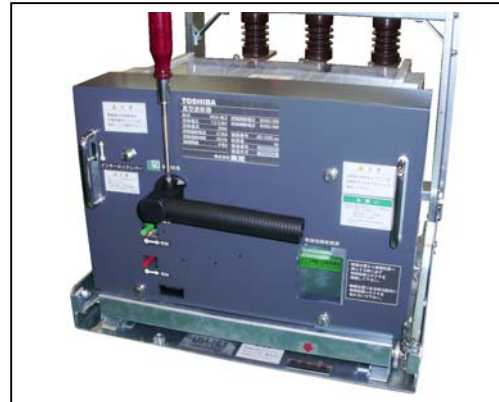
Figure 12 Using the small screw (M5) provided, fasten the handle in position. The tightening torque should be 2.94 to 3.92 N-m (30 to 40 kgf-cm).
