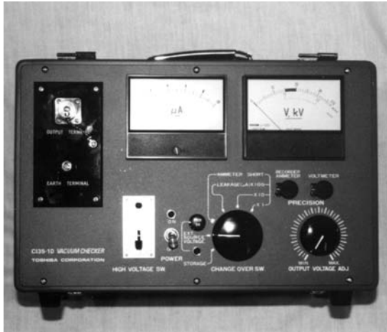
Figure 22 Toshiba Portable Vacuum Checker
