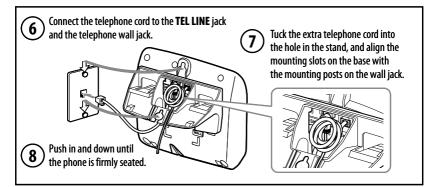
Note: To mount the phone directly on the wall, insert two 1 <sup>3</sup>/<sub>8</sub> inch, #10 screws (not supplied) into the wall using anchors suitable for the wall material. Place the screws 3 <sup>15</sup>/<sub>16</sub> inches apart, and allow <sup>1</sup>/<sub>8</sub> inch free space between the wall and screw heads.
