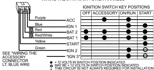
WIRING THE 6 PIN MAIN POWER HARNESS
