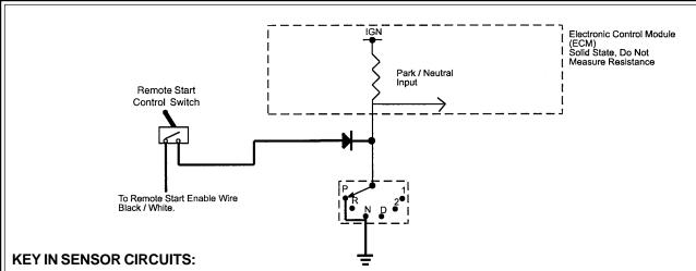
If the vehicle you are working on does not have or you cannot locate the ECM reference wire, there are two alternatives available. Although not preferred, the vehicle Key In Sensor may be reconfigured to allow a margin of safety and will prevent the vehicle with a Mechanical Neutral Start Switch from starting in gear.
