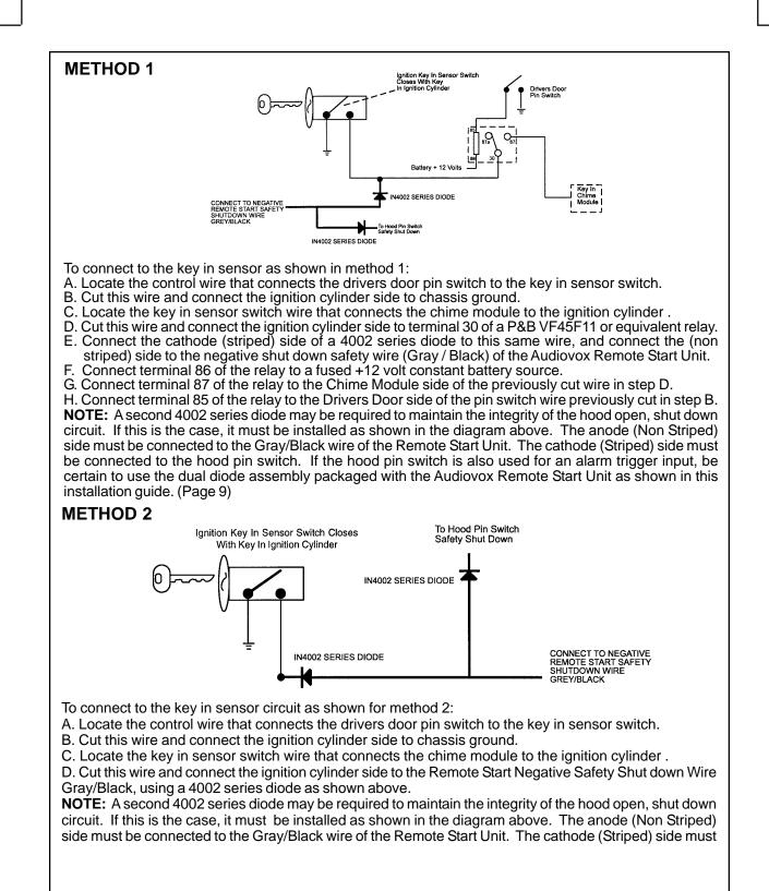
be connected to the hood pin switch. If the hood pin switch is also used for an alarm trigger input, be certain to use the dual diode assembly packaged with the Audiovox Remote Start Unit as shown in this installation guide. (Page 9)
