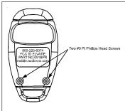
After removing the two #0 point phillips screws shown, pry apart case with the edge of a finger nail or a small common screwdriver. Keep hold of the metal key ring loop to prevent it's loss as it will separate from the transmitter case.
