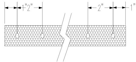
3) Use soldering iron, if necessary, to melt holes in closed strap, as shown.
