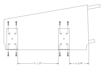
2) Use soldering iron, if necessary, to melt holes in open strap, as shown.
