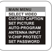
2. Press either CHANNEL up or down buttons to select the function.
