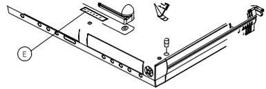
***Important Note: Before reassembly the LCD screen from Undercounter unit to a countertop unit remove the powercord to avoid damages!***
