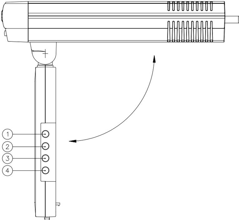
1. **MENU Button** – When pressed, the LCD control MENU is displayed.
