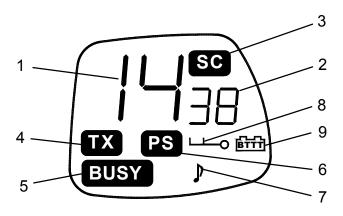
The FR-140 is equipped with an LCD display to indicate its settings and functions. The Display incorporates automatic backlighting to allow it to be seen in the dark. Pressing any of the buttons except the PTT (Push-to-Talk) button, will illuminate the display. The display will remain lit for 5 seconds after any of these buttons is pressed.
