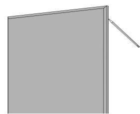
2 Install four impaling clips within marked B22 ProPanel location using drywall screws. Exact placement of each clip is not necessary.
