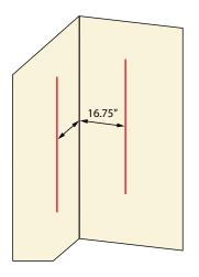
While continuing to hold panel in place, install one finish nail though the fabric face and the hardened edge of the **CT45**. Do not hammer nail completely flush with the face of the panel. Make sure finish nail is installed perpendicular to the wall surface. Repeat in each of the four corners.
