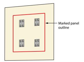
3 Start the **B22 ProPanel** 5/8" above its intended final height and press downward at a 45° angle until the panel is flush with the wall or ceiling surface.
