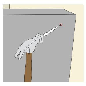
Once the finish nail has been countersunk into the panel, there may be a small hole remaining in the fabric covering. Simply scrape the fabric in this area with your fingernail and the hole will completely disappear.
