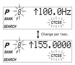
4. Press E to program the tone with the frequency stored in the channel.
