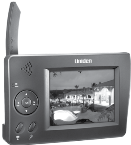
Portable receiver with 3-inch color LCD display
