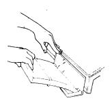
To remove the screen, open the lid and pull the screen straight out. Roll the lint off the screen with your fingers. **DO NOT rinse the screen or wash it.** Wet lint is hard to remove.
