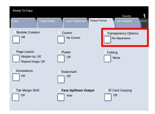
When you select the **No Separators** option, your transparencies will be delivered to the output destination **without** a blank sheet of paper separating each transparency.
