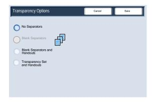
The **Blank Separators and Handouts** option will insert a blank sheet of paper between each printed transparency. In addition, a distribution set of copies will also be printed on the stock you specify using the **Paper Tray Settings** button.
