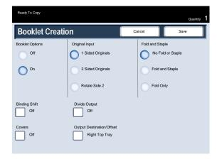
4. In addition to folding and stapling, you can also include a **Binding Shift**, or **Divide Output** (sub-dividing a large booklet into subsets) on the Booklet Creation screen.
