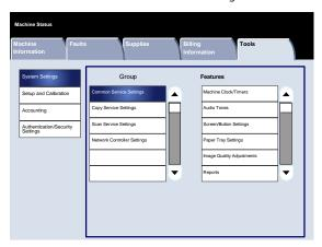
The **Setup and Calibration** menu allows administrators to access settings for **Stored Programming**, **Job Flow Sheets**, and **Paper Tray Attributes**. This screen also provides access to a calibration tool for optimizing the quality of copy and print jobs.
